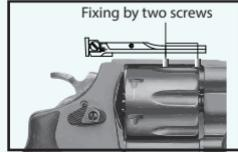
After having disassembled the standard sight, the TXT has to be fitted on the gun by means of two screws supplied into the blister pack
