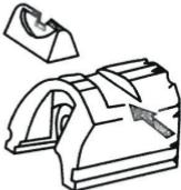
Remove existing rear sight. (Arrow direction is reversed for Colt pistols and other USA made pistols).\*
