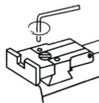
After having made the alignment with the front sight, tighten the locking screw with allen wrench.
