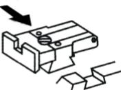
Insert the new rear sight as the arrow shows. Dovetail is tapered.
